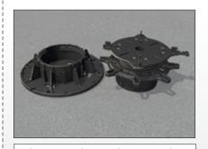
TL5 tile support from 14 cm up to 103 cm offer the same features as TL4, but can only be used in combination with TL6 coupling tubes. TL6 is cut to the required length and inserted into the guides at the top and bottom. The support disc can be adjusted by a further 4 cm by screwing.
