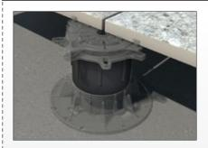
TL4K coupler 7 cm can only be used in combination with TL4 - unscrew the base plate at TL4 and insert the coupler. The height regulation of 7 cm can be adjusted as in TL4 by the central adjustment ring. This achieves a raising height of 13 to 20 cm.
