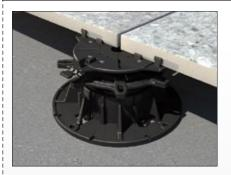
TL4 tile support 6 cm to 13 cm is adjusted by means of an adjustment ring. If necessary, fine adjustment and slope compensation is completed along with the TL3 adjustment shims 1 mm. For raising heights just over 13 cm, TL1 tile support 1 cm can also be used for the construction.
