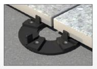
TL1 tile support 1 cm can be laid on any kind of sealing foil. The hard-wearing special plastic composite does not harden and reduces footfall sound. TL1 are stackable and can be used for raising heights from 1 cm to more than 20 cm..
