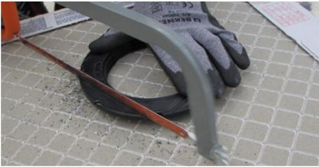
10. Turn the base upside down and remove one of the sides along the marked line.
