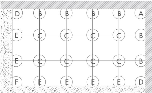
Example of an installation diagram for a rectangular terrace, open on two sides and enclosed by walls on two sides. The letters in the diagram indicate the type of pedestal. Pedestal installation instructions are described below. The installation must be **closed** on all sides by either walls or specific perimeter enclosing systems (clips or profiles).
