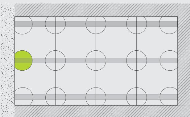
Installation plan for rectangular terrace closed on three sides.
