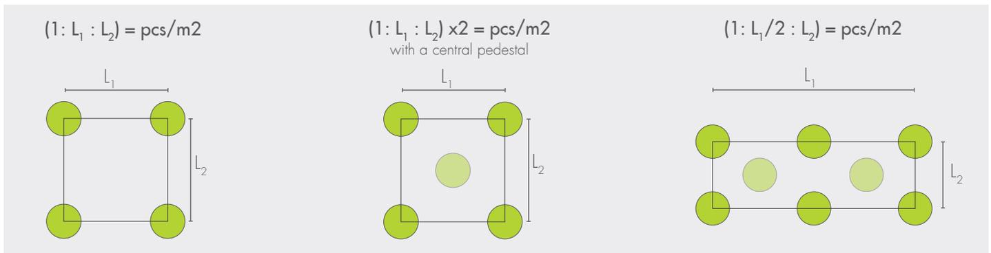
**PLEASE NOTE:** The formula does take into consideration perimeter pieces. For a precise calculation, add the number of pieces per square meter to half of the pieces resulting from the perimeter calculation.
