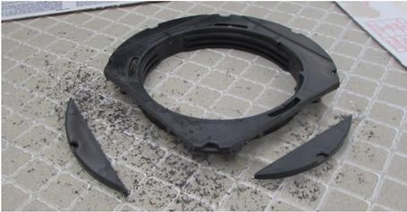
19. Turn the base upside down and remove two sides along the marked lines.
