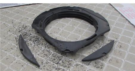
15. Turn the base upside down and remove two sides along the marked lines.
