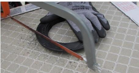
23. Turn the base upside down and remove one of the sides along the marked line.
