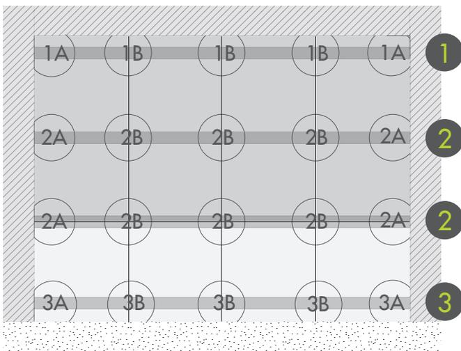
Installation diagram for a rectangular terrace enclosed on two sides. The letter specified indicates the type of pedestal, of which the installation process will be explained below.
