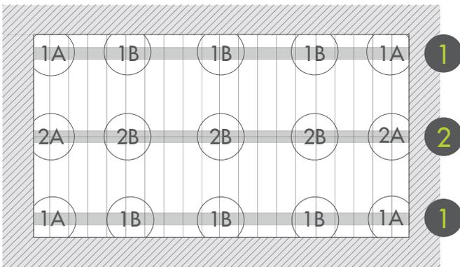
Installation diagram of a rectangular terrace closed on four sides. The letter specified indicates the type of pedestal, of which the installation process will be explained below.
