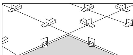
**en** When laying large tile sizes, there is a risk you will encounter differences in floor level. To offset uneven areas, we recommend using levelling spacers to guarantee a rapid and accurate fitting of the floor tiles in all conditions.
